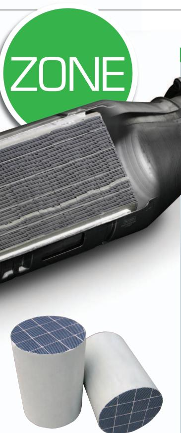
Diesel particulate filters (DPFs) are seen by many as a solution to meet LEZ standards, but others argue that their performance is affected by congestion, preventing optimal operating temperatures from being reached
